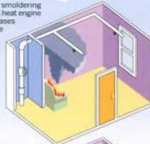
**2** As soon as the trigger mechanism is heated to the required temperature, it trips and the water is released. The immediate cooling of the heat source usually prevents other sprinkler heads from activating. Often, one or two sprinkler heads are enough to control a fire.
