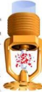
**3** The plug is forced out by the pressurized water behind it and deflected away by a beveled edge. The water sprays over the deflector plate which is designed to distribute it in an even pattern. Water will continue to flow until the main valve is shut off.
